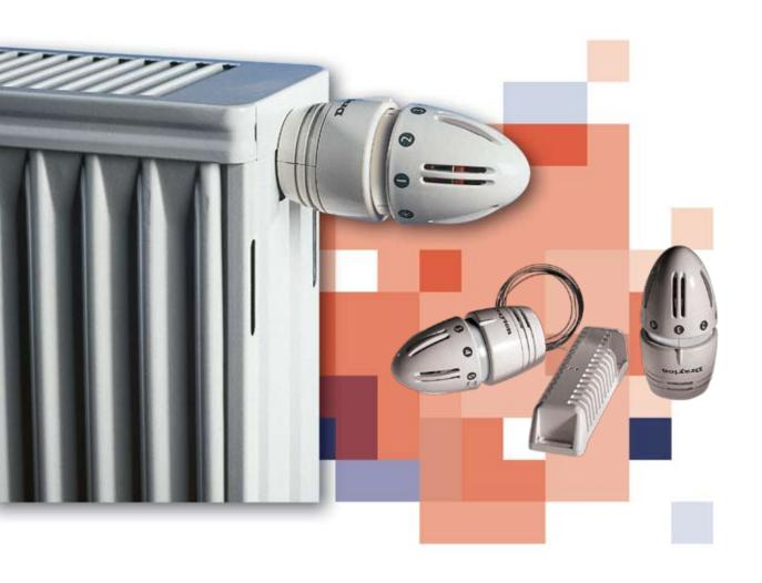
The ET40 range of thermostatic heads combine over 30 years of Drayton manufacturing expertise and reliability with innovative styling. Both the integral and remote sensing heads utilise the standard M30 x 1.5 ring nut and can be fitted to most compact radiators and thermostatic valve bodies. A full range of Drayton EB valve bodies are available, providing highly accurate room temperature control.
